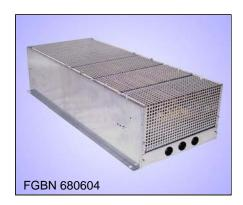
Wirewound lamina type fixed resistor, degree of protection IP  $20^{\circ}$  in fixed condition, in zinc plated steel sheet enclosure with ceramic insulated flat terminals up to 35 A and ceramic insulated bolt terminals for higher currents inside the device. With drillings for 3 cable entry points PG 13,5, which are closed by rubber sockets.
